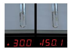
**High-temperature microemulsions**: By replacing water in microemulsions by a room-temperature ionic liquid, the thermal stability range of microemulsions can be enlarged. Microemulsions with ethylammonium nitrate as polar phase exhibit a thermal stability ranging from 30 up to 150 °C at ambient pressure.
